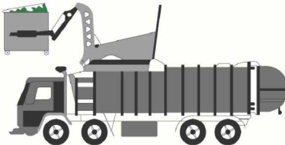
Front-lift-loading waste collection vehicle
